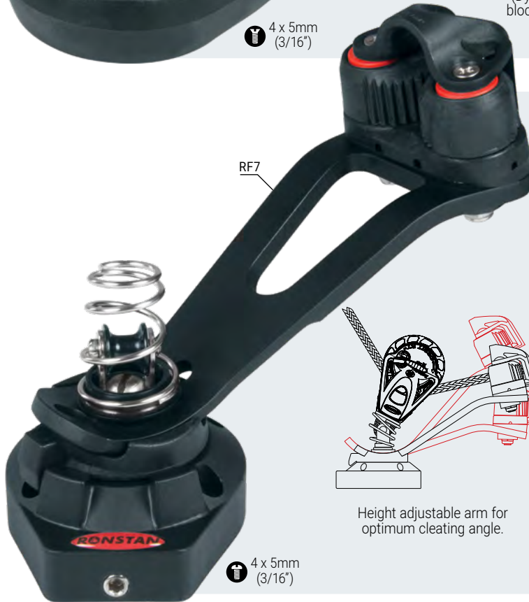
Twin ball bearing races minimise friction. Adjustable ratchet system prevents the arm from falling to leeward.
