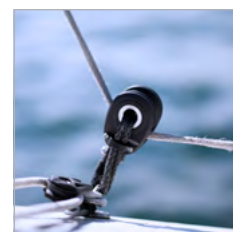
Cheek plates twist to open block
